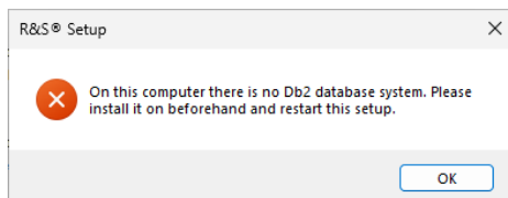
Figure 2.24 The DB2 database system must be installed first.
